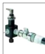
Connect the sample syringe directly to the purge and trap valve via the integral male luer fitting
