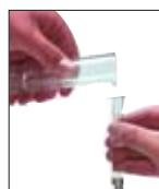
Easily remove the syringe plunger and load water sample into the syringe barrel
