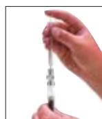
Add an internal standard or surrogate sample directly to your sample through the twist valve with a 10 μL syringe
